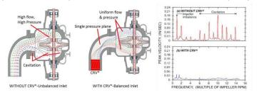
**Problem-Pump & Check Valve Vibration:** Check valves, respond to flow and pressure disturbances. Such turbulence cause the pin to fail, leakage though the pin starts, and the valve seat will not seal. CRV® installation reduced the noise, extended seal, bearing, impeller life, increased delivered head and flow.
